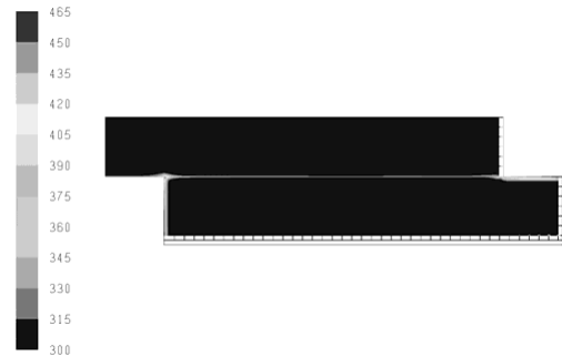
Figure 8. Temperature distributions in the gob areas after about 9 days (with 0.75 in. pressure drop at regulator 2).
