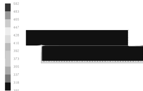
Figure 10. Temperature distributions in the gob areas after about 9 days (with permeability decreased 10 times).
