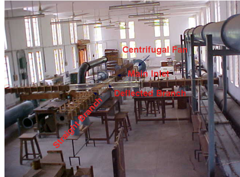
Figure 2: Laboratory setup for testing the flow in junctions and splits.
