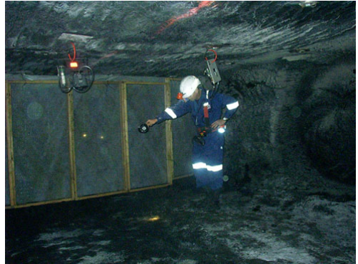
Figure 3. Filter panel installation and dust and air velocity measurements during field testing of the air filtration concept at a southern Illinois mine.
